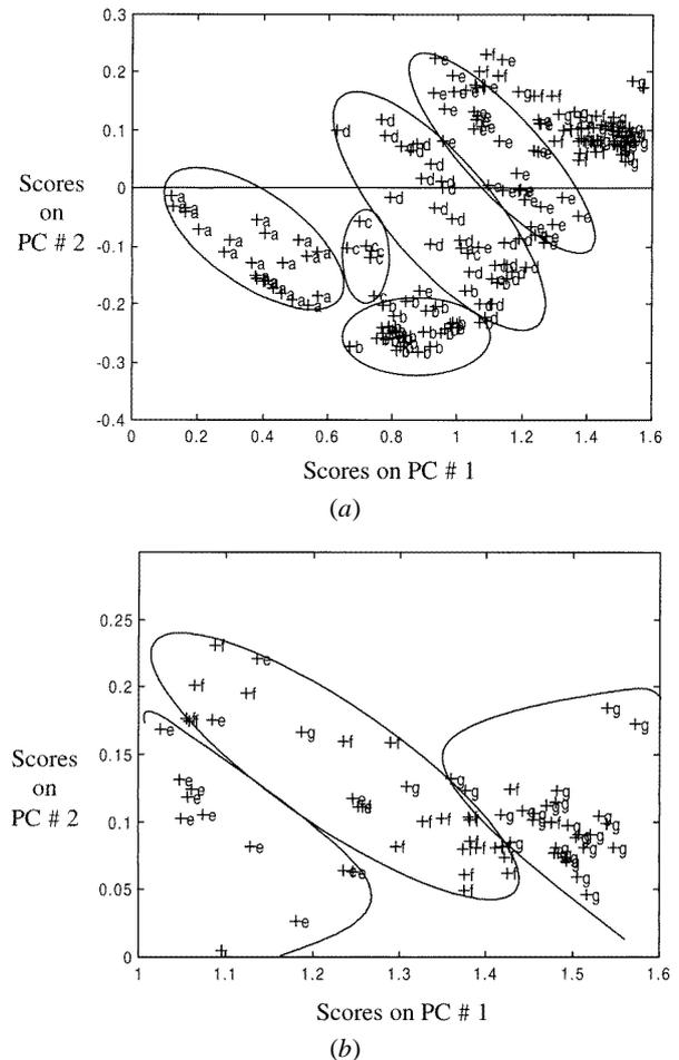
**Figure 2.** (a) Results of the principal-components analysis of the response of a four-element tin-oxide sensor based electronic nose to the bananas' aromas. Seven clusters or categories appear. These correspond to seven states of ripeness. (b) A detailed expansion of an area of (a), showing the boundaries corresponding to categories e, f and g.
