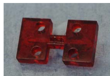
Figure 6: Picture of the MSL cell showing the small liquid reservoir (centre).
