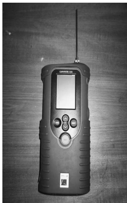
Fig. 2. Typical Cyrano 320 e-nose which contains 32 carbon black conducting polymer composite sensors.
