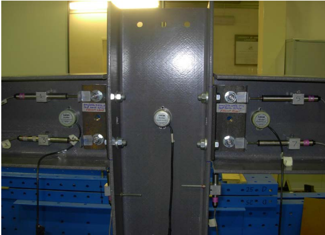
Fig. 5. Details of nominally pinned beam-to-column joint test Wmj254_2M16_ST1-1.
