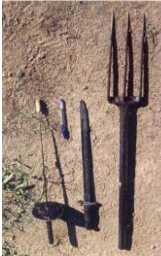
NPA's demining probes
