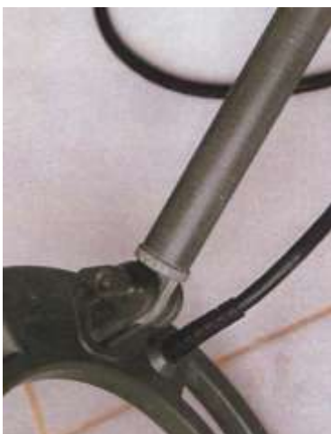
The Schiebel's weak hinge between head and pole
