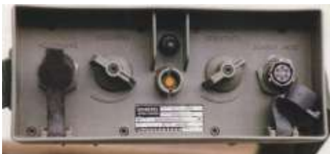
The Schiebel control box
