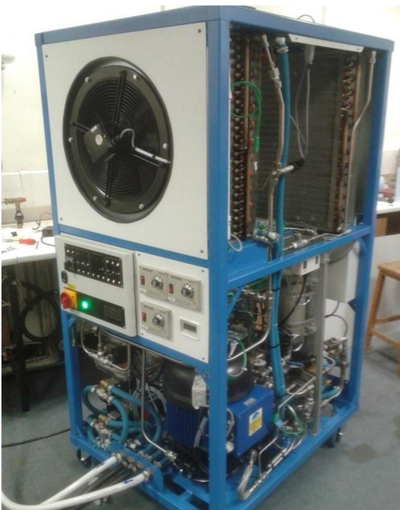
8 kW cooling capacity prototype
