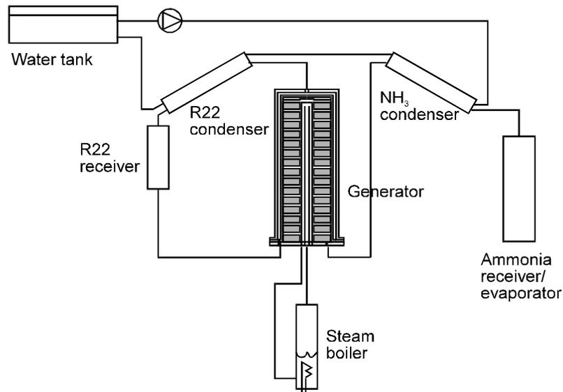
Figure 2: Schematic of heat transfer test rig
