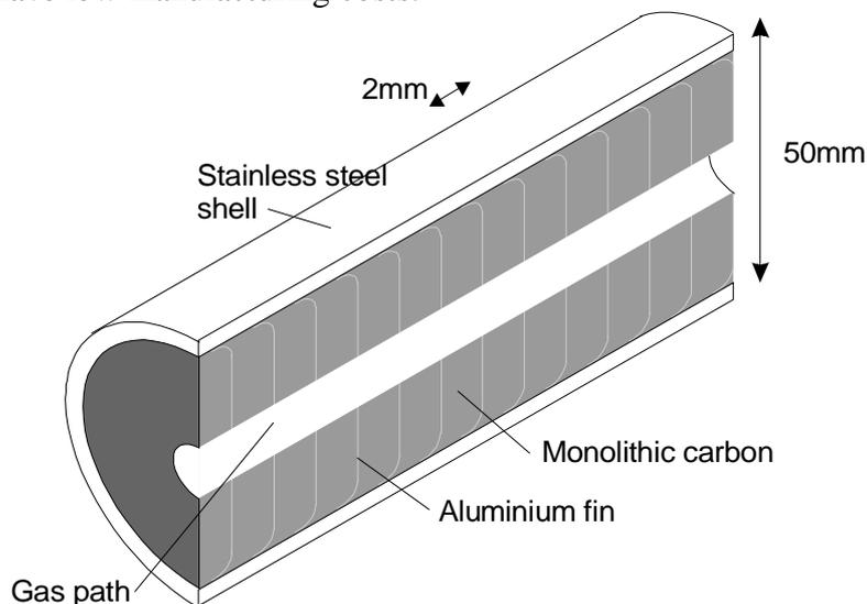
Figure 5: Generator design configuration
