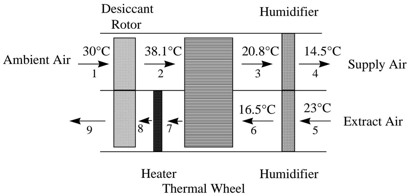
Figure 6: Schematic desiccant cooling system
