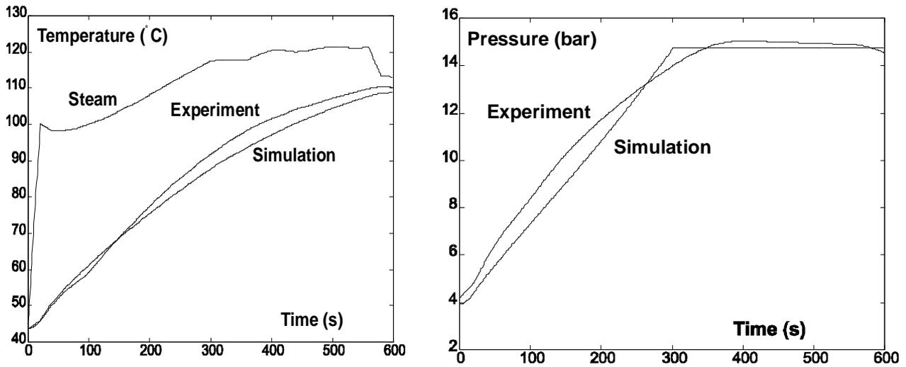
Figure 4: Experimental and simulated generator conditions
