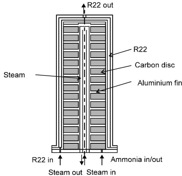
Figure 3: Cross section through generator
