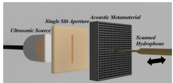
Fig. 11. Schematic diagram of the image resolution experiment at 300 kHz. This used an aperture test plate that was placed between the ultrasonic source and the metamaterial, next to the latter's surface. The miniature hydrophone receiver was then scanned in a horizontal line parallel to the output surface of the metamaterial. The ultrasonic source, slit aperture and metamaterial were held stationary during this measurement.
