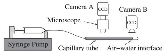
FIG. 1. Sketch of the experimental setup.
