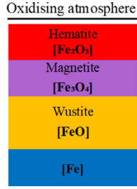
Figure 1. Schematic representation of the typical oxide scale layer that forms as part of a steel reheating process.
