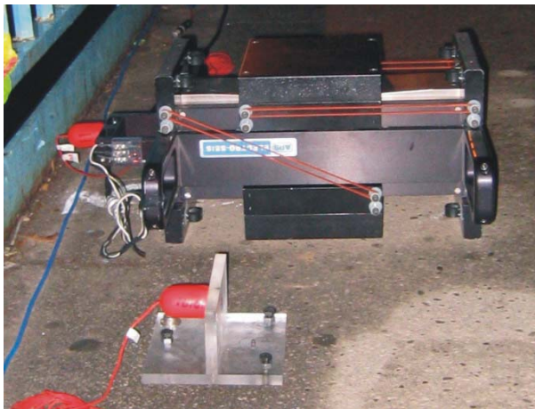
Figure 7: Electrodynamic shaker operating in the horizontal mode.
