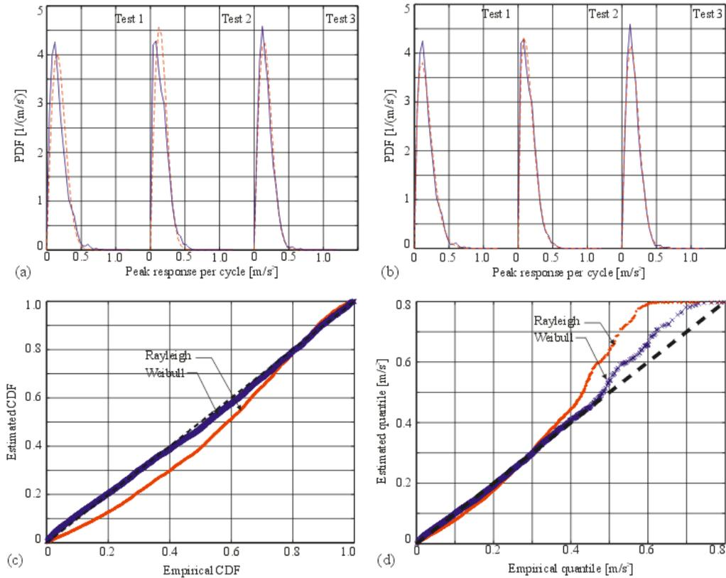
Figure 9: (a) Rayleigh and (b) Weibull PDFs for peak response per cycle in the three tests and quality of the distribution fits in Test 1 as illustrated using (c) probability and (d) quantile plots.
