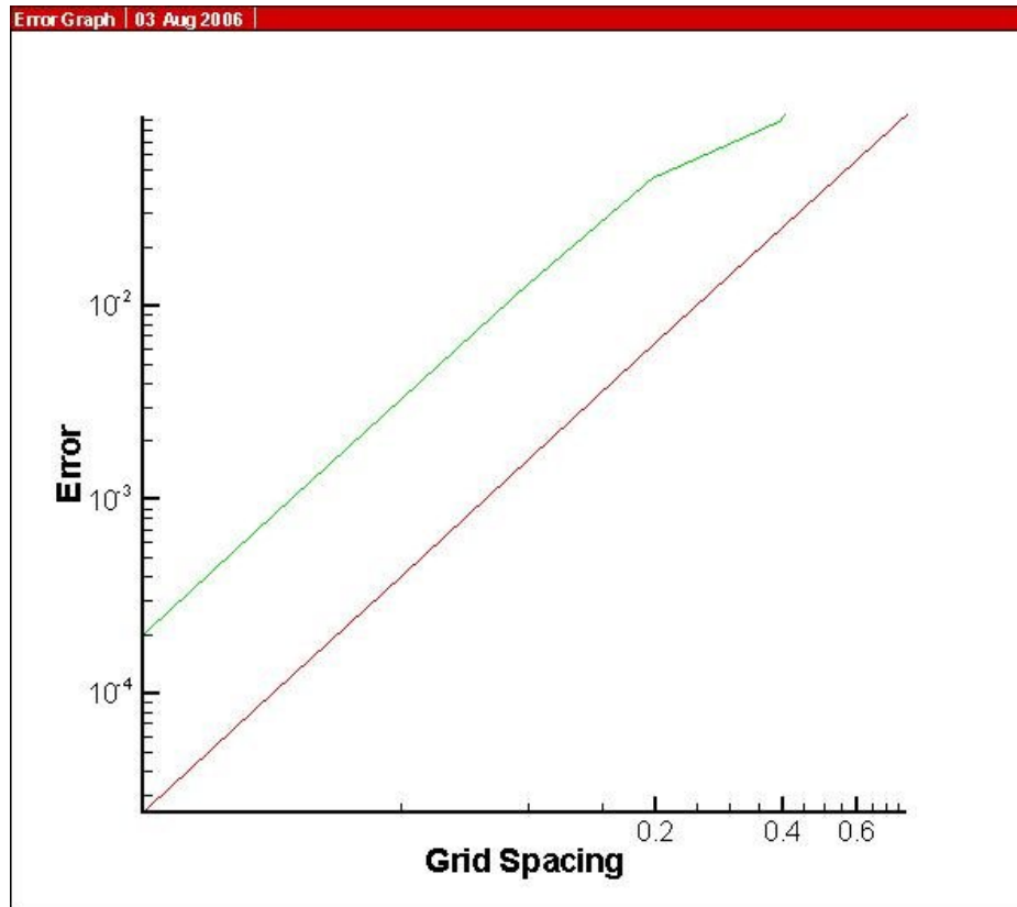
Figure5.17 : Truncation Error V.S. Grid Spacing for Second-Order Central Difference Red – Uniform Distribution Green – Non-uniform Distribution
