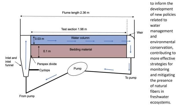
Schematic figure to illustrate custom-built recirculating flume experimental system, comprising of 3 separate units each containing 3 flumes. Each flume is 1.98 m, long, 0.1m wide and 0.2 m deep.
