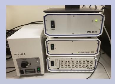
Turn on the three power switches on the stack of boxes, then turn on the HXP lamp.
