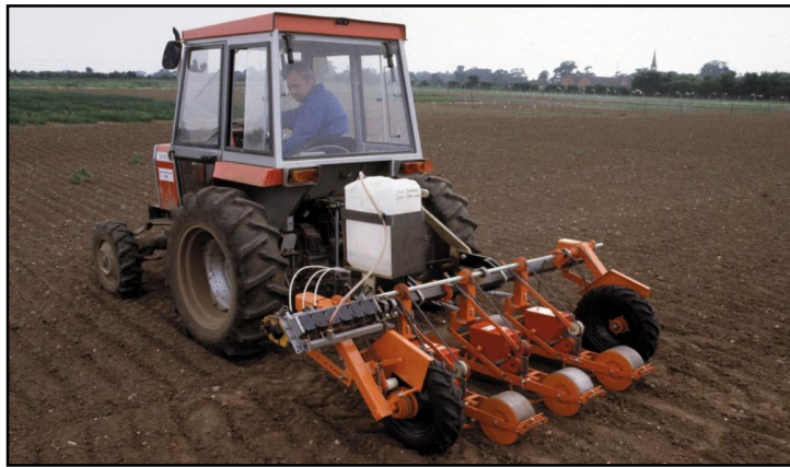
Injection of liquid starter fertilisers into the soil below crop rows
