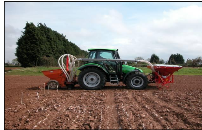
Injection of fertiliser granules into soil beside crop rows
