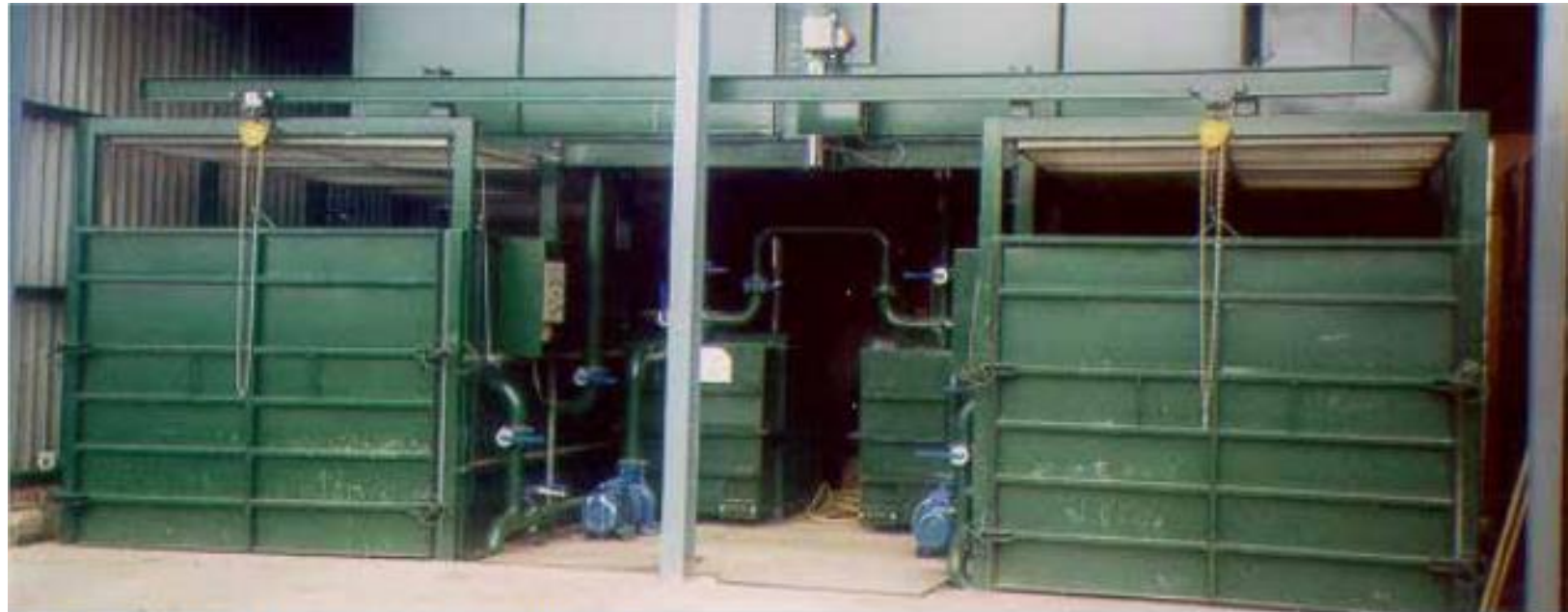
1. HWT facility with 2 x 4 tonne tanks and overhead holding tank
