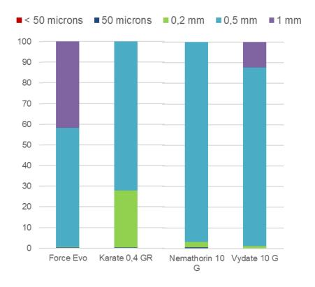
Low dust = 3-50g of dust per 100 kg of product and no granule size changes after shaking in Heubach tank
