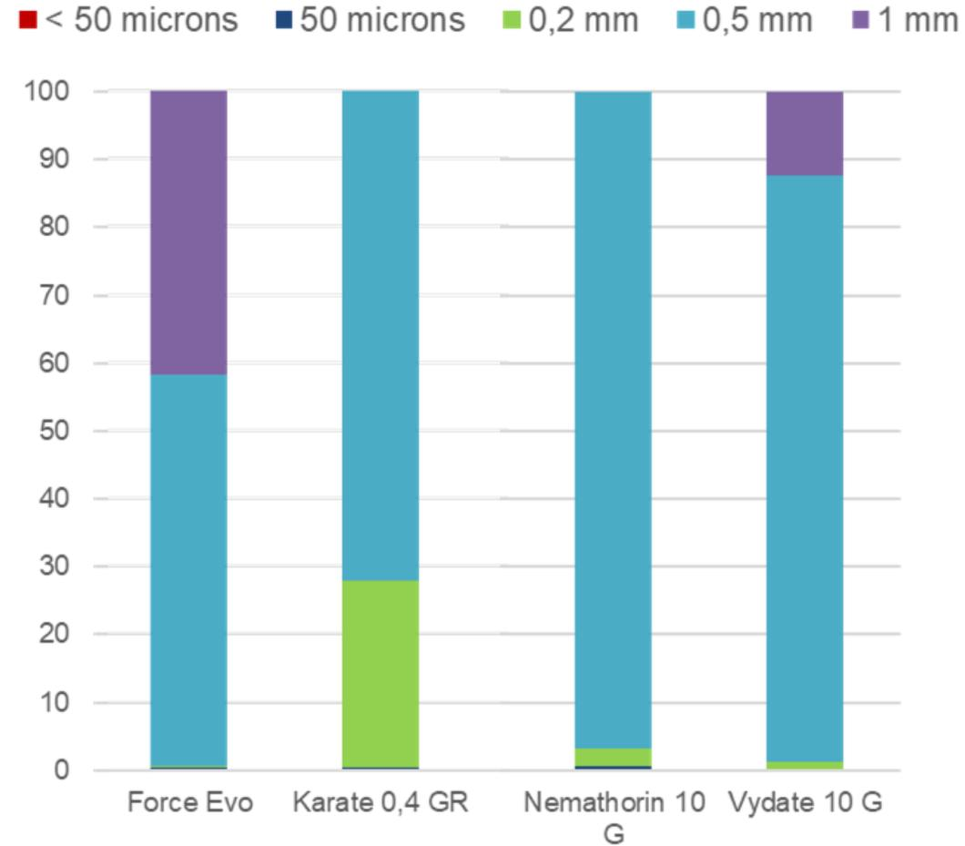
Low dust = 3-50g of dust per 100 kg of product and no granule size changes after shaking in Heubach tank
