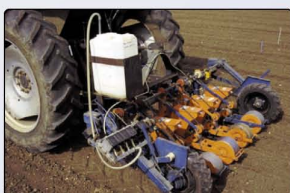
BCAs suspended in guar gum were applied in furrow using a modified drill
