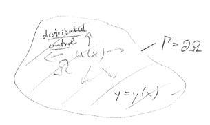
Aim: Choose the distributed control u=u(x) in se such that the stationary temperature distribution y(x) is 'close te' a sine, desired distribution /2 (4).
