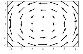
We often represent vector fields by plotting some representative vectors (arrows) in  $\mathbb{R}^2$  or  $\mathbb{R}^3$ . The above figure shows the vector field  $\mathbf{F}(x, y) = (-y, x)$  produced in Python using the **quiver** function. We plot the arrows at integer grid points in  $[-3,3] \times [-3,3]$ . Longer arrows = larger magnitude.
