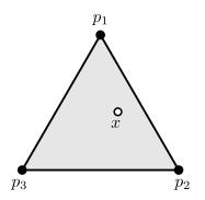
$$x = \sum_{i} \alpha_i(x) p_i, \quad \alpha \in \Delta_n := \{ \alpha \in [0, 1]^n \mid \alpha_1 + \dots + \alpha_n = 1 \}.$$
