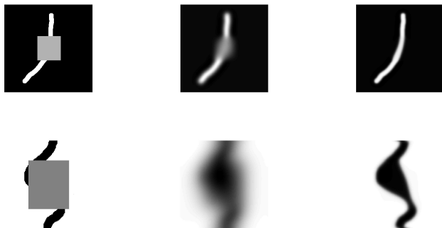
Figure: Cahn-Hilliard inpainting in two steps, namely with \epsilon = 0.1 and \epsilon = 0.01 (i.e. \epsilon = 1.6 and \epsilon = 0.01 )
