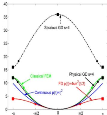
The viscous approach will work while the two-grid one will hardly do it because of the uncertain location of the pathological points in dispersion curves.
