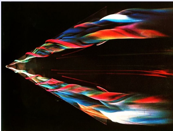
Figure: Vortices on the upper surface of a thin Delta wing. Henri Werl, ONERA. e-fluids Gallery of Images.
