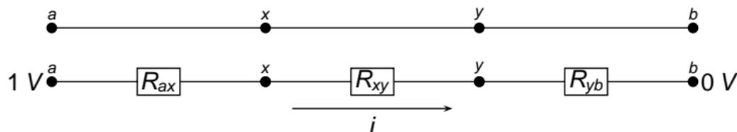
**Electric resistor network:** the voltage  $u$  is **harmonic** ( $C = 1/R$ ):
