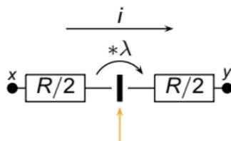
**Voltage amplifier:** keeps the current, multiplies the potential.
