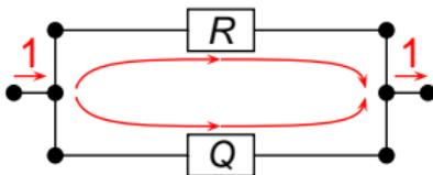
The physical unit current is the unit flow that minimizes the sum of the ohmic power losses  $\sum i^2 R$ .
