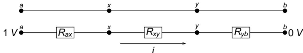
**Electric resistor network:** the voltage  $u$  is **harmonic** ( $C = 1/R$ ):
