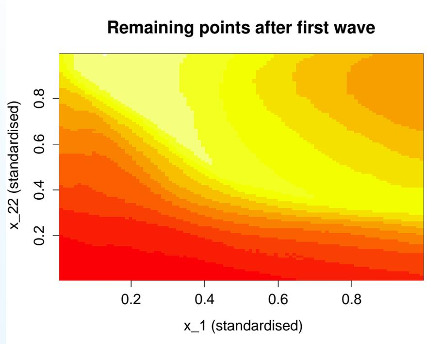
Plots such as those above illustrate the regions that history matching removes. Each point on the heatmap was generated by fixing  $x_1$  (maximum upper layer storage) and  $x_{22}$  (time delay), and varying the remaining parameters over a grid, and calculating the proportions that would be rejected by history matching. In redder areas, most points were rejected. In whiter areas, most points were accepted.
