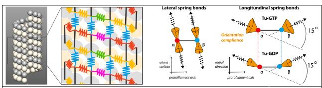
**Fig.1** Lattice of spring-bonds model. Left: a microtubule composed of tubulin dimers organised into 13 protofilaments; the pitch of the spiral is such that there is a seam on one side. The panel shows the six bonds between dimers. Right: sketch of the bonds for Tu-GDP and Tu-GTP  $\alpha\beta$  dimers which have characteristically different spring bonds. Each bond has a length, a stiffness, a 3D directional preference (cones) and a strain-dependent breaking rate.
