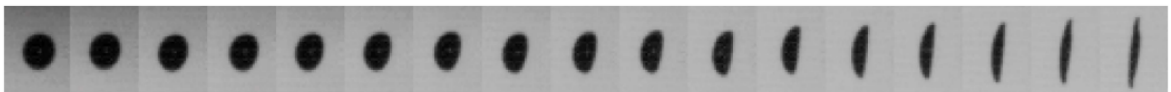
Figure 2: Drop deformation evolution 2 for a reference velocity of 90 m/s and an initial drop radius of 524 \mu\text{m} .
