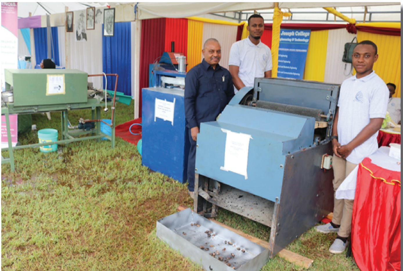
The Director of Innovation and Technopreneurship Acceleration Facility at St. Joseph University in Tanzania (SJUIT) Eng. Dr Lawrence Kerefu (in black shirt) with fourth-year engineering students who developed a mobile automatic cashew-nut shelling machine shown in the picture as one of the projects in fulfilment of the requirements for the degree of Bachelor of Mechanical Engineering.
