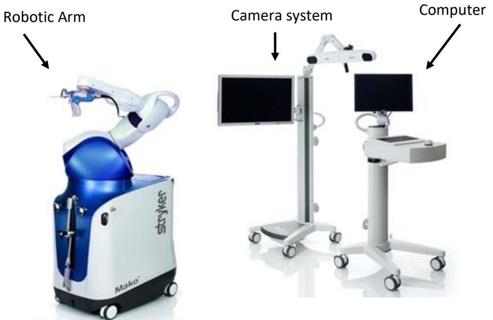
Picture 2. The parts of a robotic system for knee surgery
