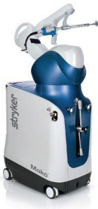
Figure 1: The MAKO robot. The surgeon moves it into the surgical field after exposure of diseased joint and the robot controls the preparation and insertion of the implants
