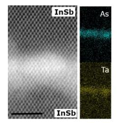
Initial TEM results on InSb/TaAs/InSb (001) heterostructure growth by MBE. Left: electron image of TaAs layer embedded in InSb (scale bar 5 nm). The TaAs atomic structure is not well resolved in its ultrathin film form, but the typical InSb "dumbbells" are clearly resolved in both the substrate and MBE-grown epitaxial overlayer. Right side panels (not to scale) show the EDX signal for As and Ta, confirming confinement of these elements to the ultra-thin layer.
