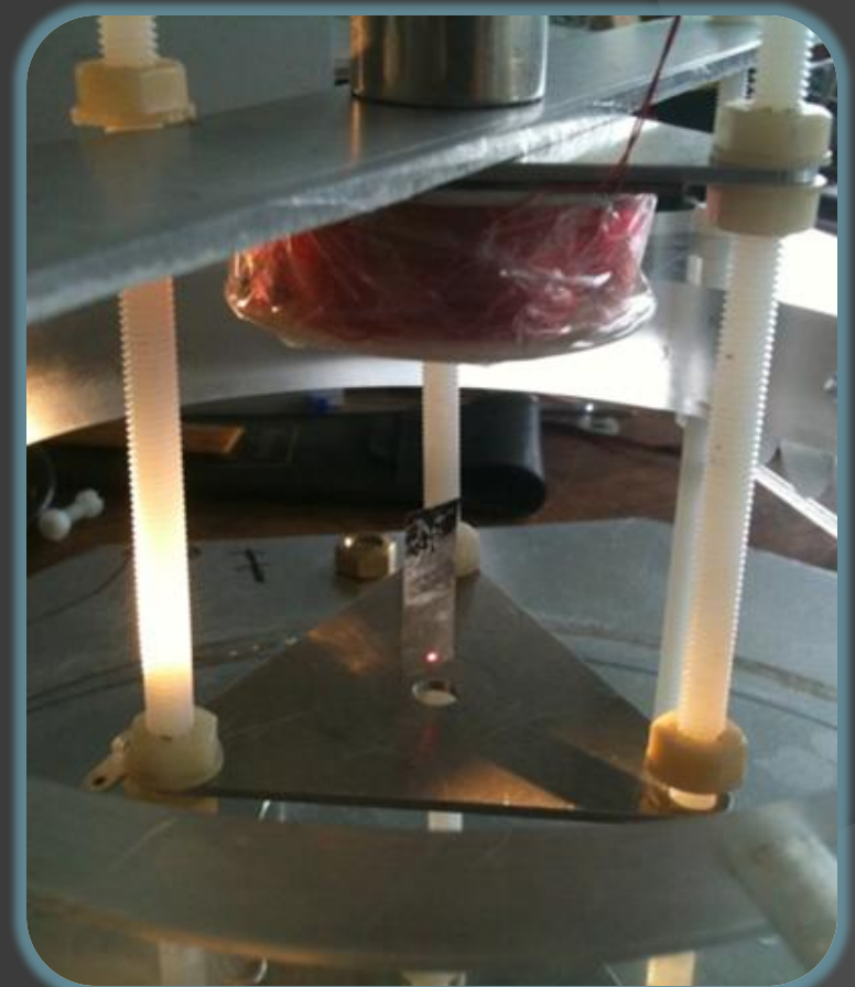
Fig 4. Photograph of floating dummy Nickel sample in the current experiment.
