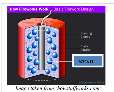
This diagram shows the basic structure of a firework. The key components that determine the colours we see are packed inside the **stars**. These pellets contain metal salts, or other compounds, that emit different colours when ignited.
