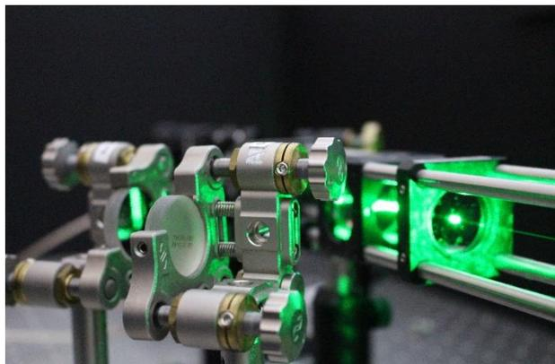
We send in green light to excite a single NVC, polarizing its electron spin, before using magnetic resonance to control its quantum state and then detecting its final state by detecting the red fluorescence it emits.
