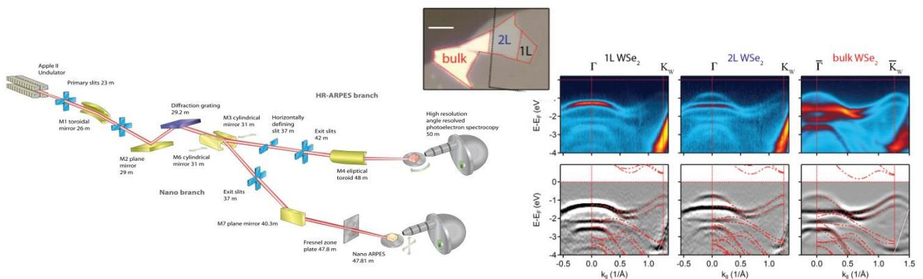
(left) Schematic of the I05 beamline at Diamond Light Source; (right) example nanoARPES results from a 2D heterostructure, showing layer-dependent valence band structure in the 2D semiconductor WSe<sub>2</sub>.
