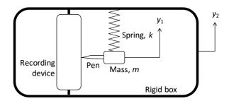
A seismic wave moves the box vertically so that its height as a function of time is given by  $y_2 = a_s \cos(\omega t)$ .
