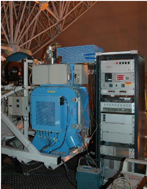
HARP on the JCMT 16-pixel heterodyne array receiver
