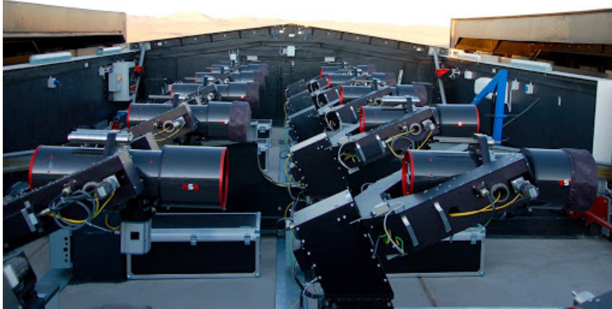
Figure 1.14: The NGTS telescopes in the enclosure at Paranal. Ten of the twelve can be seen, with the other two located behind the camera. This photo was taken by Dan Bayliss, and obtained through private communication.
