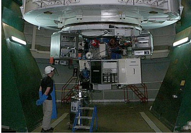
Figure 2.11: ISIS: A two channel intermediate dispersion spectrograph. Shown mounted at the Cassegrain focus of the William Herschel Telescope.
