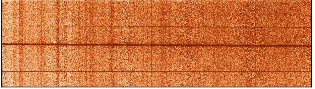
Figure 3.5: Typical (raw) 2D spectrum of a source observed with ISIS on the WHT. The x axis corresponds to the spectral direction whereas the y -axis is the spatial direction. The latter is always aligned with the slit. The black horizontal lines indicate the spectra of observed stars whereas the dark vertical lines correspond to sky lines.
