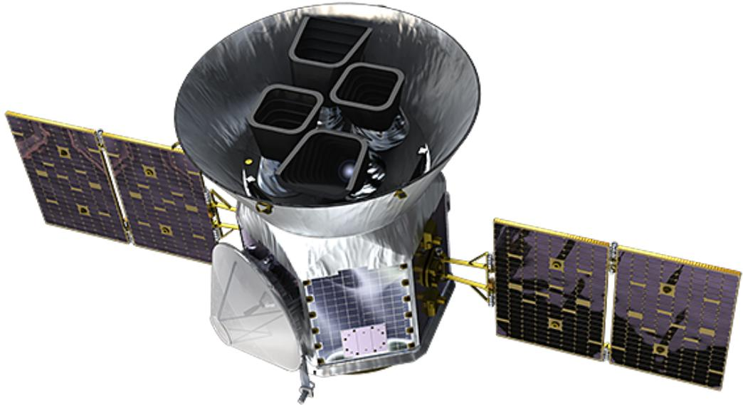
Figure 1.12: *TESS* telescope showing the arrangement of its 4 cameras, solar panels, sun-shade and downlink antenna. Figure from <https://TESS.mit.edu/>
