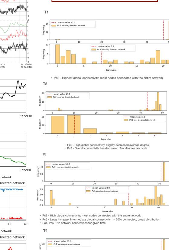
· Pc2 - Highest global connectivity, most nodes connected with the entire network Pc3 - Overall transition to lower connectivity Histograms of frequency vs network degree got the nonzero lag directed network. Sub-
