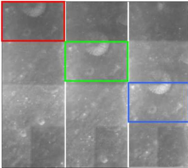
Figure 28: The AMIE camera on board SMART-1 has three fixed-mounted filters which see the Moon in different colour bands. The figure shows four consecutive images taken by AMIE from left to right. The fixed filters are indicated by coloured frames. The images, taken only a few seconds apart, show how the surface is moving through the different filters. Credits: AMIE Team
