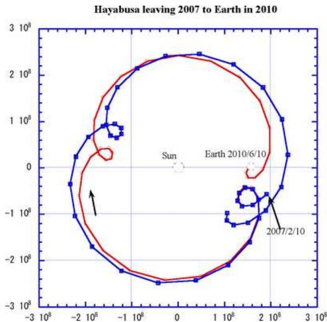
Figure 31: *New trajectory (red line) leaving Itokawa vicinity in spring of 2007, returning to Earth in June of 2010 is shown here. The Xenon gas consumption meets the current amount that remains. There will be some strategy needed and left for the operational discussion on how the attitude is protected against unexpected disturbance.*
