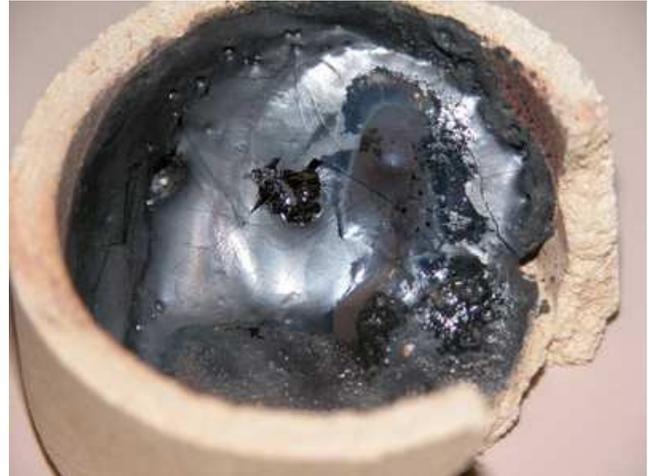
Figure 26: Slag—a low-oxygen byproduct of Cardiff's device. Slag may prove useful as a raw material for bricks, pavement or radiation shielding.
