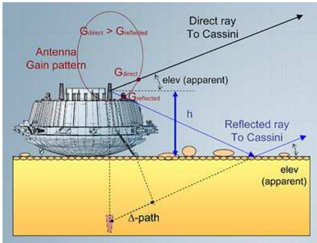
Figure 6: This technical sketch illustrates the radio signals emitted by the Huygens probe from Titan's surface after touch down on 14 January 2005. The probe survived the impact and continued to transmit to the Cassini mothership,
