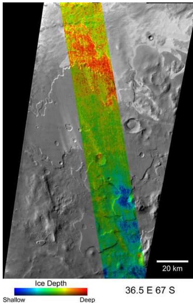
Figure 5: This color-coded map indicates the depth to icy layers at a site in southern Mars. The dense, icy layer retains heat better than the looser soil above it, so where the icy layer is closer to the surface, the surface temperature changes more slowly than where the icy layer is buried deeper. Image credit: NASA/JPL/ASU
