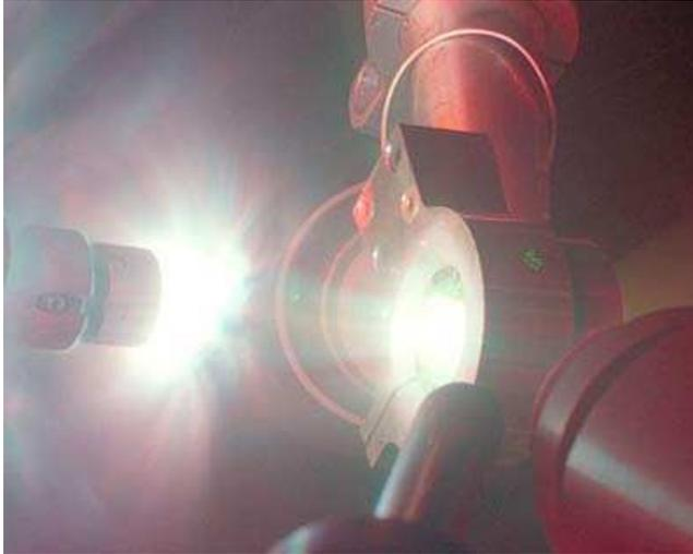
Figure 6: A laser vaporizes a diamond cell, inducing a shock wave that produces pressures over 10 million times atmospheric pressure, greater than the pressure at Earth's core. The experiment was conducted at the Omega laser facility operated by the University of Rochester in New York. (Raymond Jeanloz/UC Berkeley)
