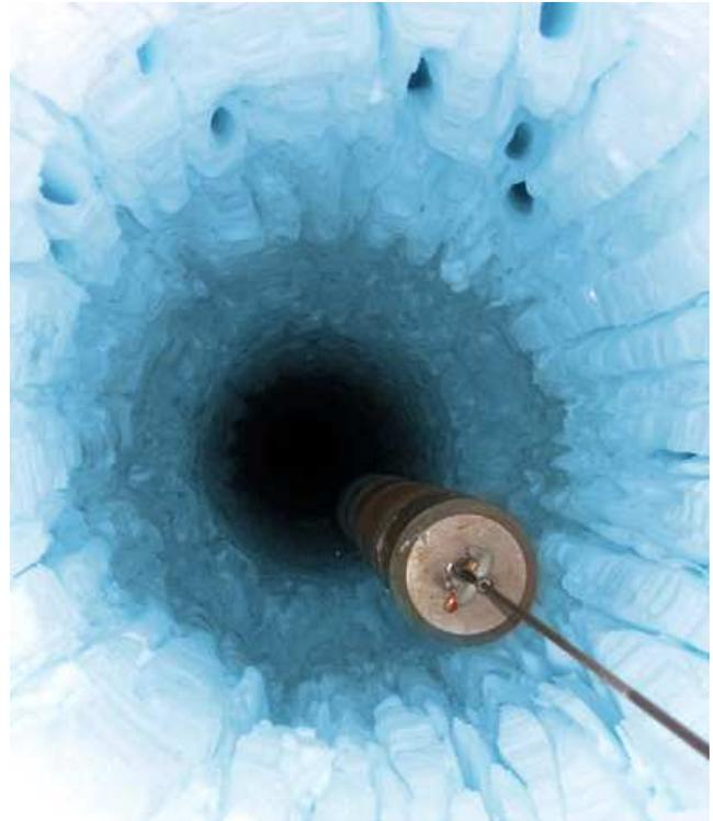
Figure 33: *The telescope's optical detectors are deployed in mile-and-a-half deep holes in the Antarctic ice.*
