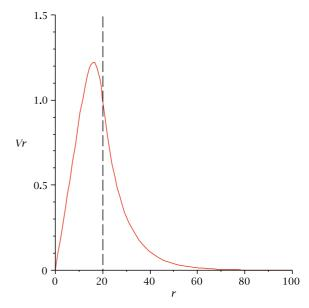
**Fig. 7.** The amplitude of the radial velocity,  $v_r(r)$  in r, for case B. Here  $v_r(r)$  is made dimensionless by  $v_{A0} = 2 \times 10^8$  cm/s and r by the ion gyroradius,  $\rho_i = 27$ , cm both taken at r = 0. The dashed line marks the boundary between the interior and exterior of the current thread.
