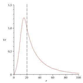
**Fig. 4.** The amplitude of the radial velocity,  $v_r(r)$  for case A. Here  $v_r(r)$  is made dimensionless by the Alfvén velocity,  $v_{A0} = 2 \times 10^8$  cm/s, and r by the ion gyroradius,  $\rho_i = 27$  cm, at r = 0. The dashed line shows the boundary between the interior and exterior of the cylinder.
