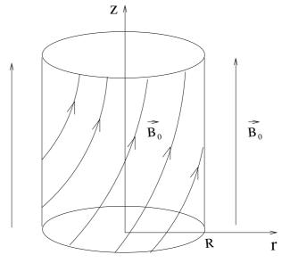
**Fig. 1.** Model of a current thread. The plasma density is constant everywhere, but the magnetic field is changing, such that it is straight at r = 0, then it twists, and then it is straight again at  $r \ge R$ .
