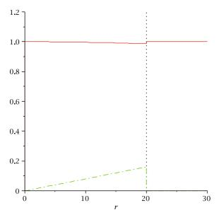
**Fig. 5.** The plot of  $B_{0z}$  (full line) and  $B_{0\varphi}$  (dashed-dotted line) fields in the interior and exterior of the tube for case B. The magnetic field is made dimensionless by the magnetic field at r = 0, 50 Gauss, and r by the ion gyroradius at r = 0,  $\rho_i = 27$  cm. The expressions for the magnetic field components are given by Eqs. (32) and (33). The dotted line marks the boundary between the interior and the exterior of the current thread.
