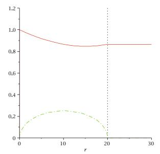
**Fig. 2.** The plot of  $B_{0z}$  (solid line) and  $B_{0\varphi}$  (dashed-dotted line) fields in the interior and exterior of the current thread for case A. The magnetic field is made dimensionless by the magnetic field at r = 0, (50 Gauss); r is expressed in units of ion gyroradius at r = 0,  $\rho_i = 27$  cm. The expressions for the magnetic field components are given by Eqs. (28) and (29). The dotted line marks the boundary between the interior and the exterior of the tube.
