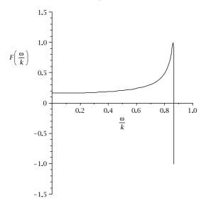
**Fig. 3.** The dispersion function as a function of the phase velocity,  $\omega/k$ , for the case A. The phase velocity is expressed in units of  $v_{A0} = 2 \times 10^8$  cm/s. It is obvious that the dispersion function intersects the horizontal axis in just one point, so the dispersion equation admits only one solution.
