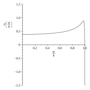
**Fig. 6.** The dispersion function  $F_2(\omega/k)$  for case B. The phase velocity  $\omega/k$  is expressed in units of  $v_{A0} = 2 \times 10^8$  cm/s. The dispersion function intersects the horizontal axis in just one point, so the dispersion equation admits only one solution.
